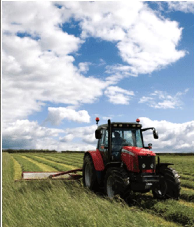
Massey Ferguson 5400 Series tractors, including this 115 hp Model 5480, are built to outlast the competition with a drive train engineered to handle 50% more power the new Tier III engines produce. The 16F x 16R Dyna-4 semi powershift transmission that is standard with 5400 Series is unique in the mid range tractor market with its clutch free shifting and three function shuttle lever.
